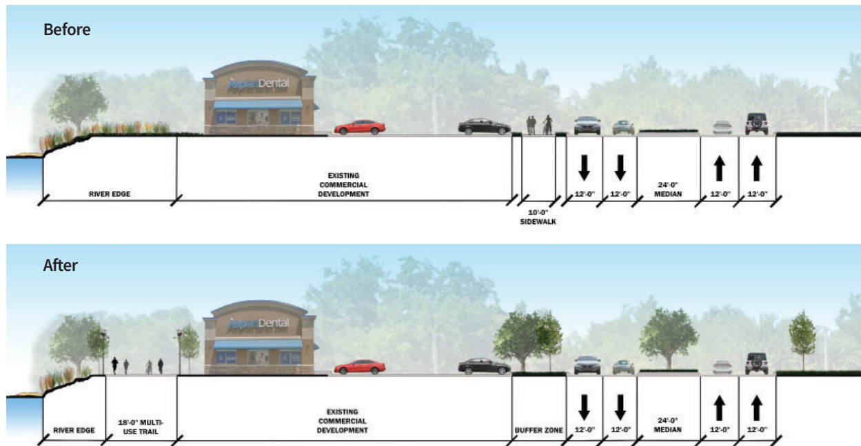
Figure 12. Before and After Images of Multiuse Trail by Commercial Area along Riverside Parkway
